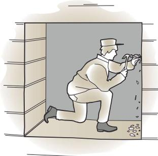
1. Hack out a work hole that is sufficiently large to insert the bottom cone just above the connector pipe.
