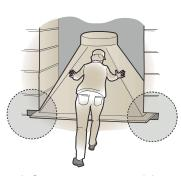
Scrape out a masonry joint so that the bottom cone can rest on the underlying stones.
