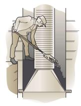
5. Cement the cone into place and lay 5-10cm of mortar over the joint between the liner and the
