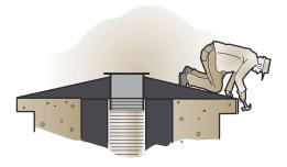
9. Install the top liner approx. 2cm above the existing concrete cone and cement with concrete from the liner. After remediation call an authorised inspector.
