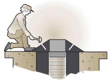
8. Brick up and seal the work hole.
