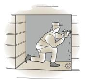
1. Hack out a work hole that is sufficiently large to insert the bottom cone just above the connector pipe.
