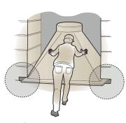
Scrape out a masonry joint so that the bottom cone can rest on the underlying stones.
