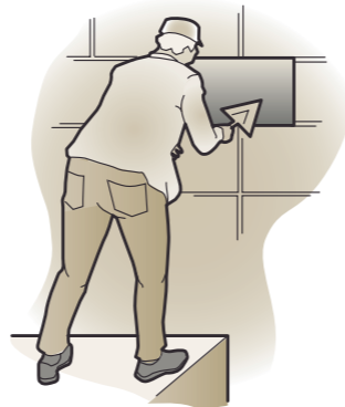
6. Brick up and seal the work hole.
