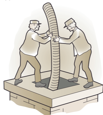
3. Insert the liner through the chimney using a draw plug.
