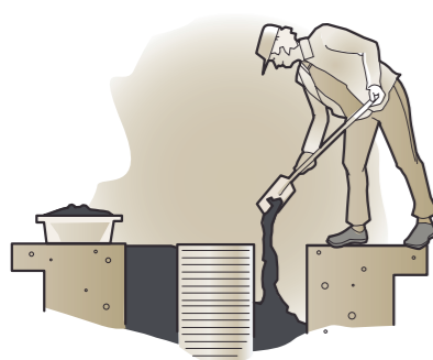
7. Fill the space between the chimney and liner with chimney insulation (Vermiculite, see page 25).
