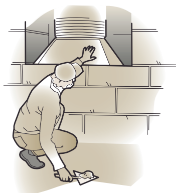
4. Assemble the bottom cone and the liner, secure using acid resistant pop rivets.
