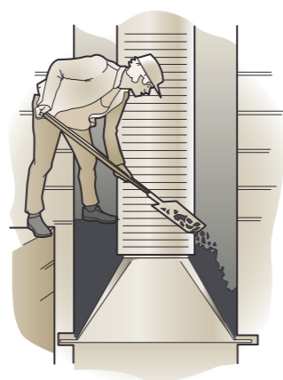
5. Cement the cone into place and lay 5-10cm of mortar over the joint between the liner and the cone.
